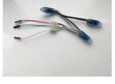
The colour of the jumper wires from the connector block is not important – it is the colour of the wires that come out of the connector block to the string that is important.
