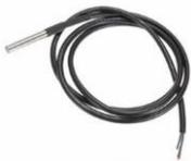
A DS18B20 waterproof temperature sensor. It has three wires at one end, and a metal sensor on the other end. This version is waterproof and the sensor can be dipped in water. A smaller, cheaper, non-waterproof version is also available.
