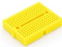
A mini breadboard. This has a top and bottom section. All the points along each column in each section are joined, so we can make electrical connections.
