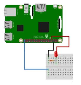
Step 6: Take 1 jumper lead and attach to E17 on the breadboard and GPIO 26 on the Pi.
