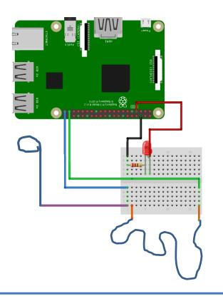
Step 9: Hook the loop you made in the short wire over one end of the bendy wire like this...
