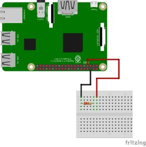
Step 4: Take the LED and insert into holes F5 and F6 on breadboard. **MAKE SURE THE LONG LEG OF THE LED GOES INTO F6.**
