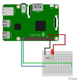
Step 7: Take 1 jumper lead and attach to A1 on the breadboard. Now take the short length of bellwire, bend the end carefully around your finger then insert the other end into the free end of the jumper lead you just attached to the breadboard.
