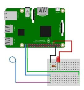
Step 8: Take the long piece of bell wire and bend it into an interesting shape. Remember – the more bends you add, the harder your game will be! Then insert the two ends of this piece of wire into A2 and A17 on the breadboard.
