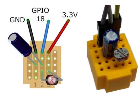
The capacitor has a short leg and a long leg. The side with the short leg also has a stripe. This is the negative (ground) side.
