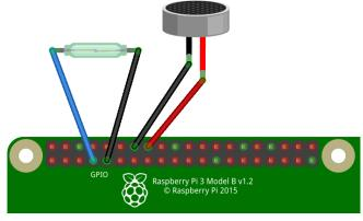
Connect the reed switch to Ground and GPIO4.
