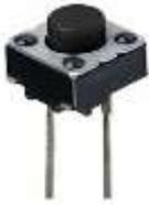
A switch can be connected any way around. When pressed, it allows electricity to flow; when released, the electricity stops. This kind of push-button is known as a “momentary press-to-make switch”.
