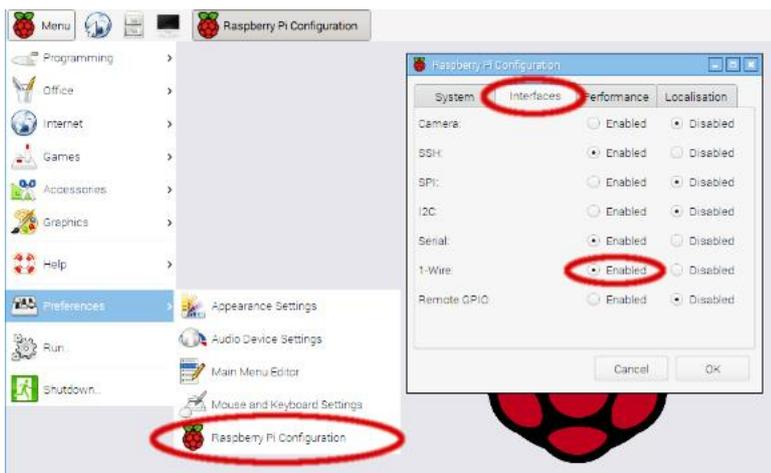
The temperature sensor uses a 1-Wire interface (positive and negative connectors, plus 1 data connector). We need to turn 1-Wire on.
