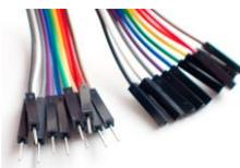
Jumper wires. You should have six male-to-female jumpers (sticky-outy at one end, inny at the other end) and one male-to-male jumper (outy at both ends).
