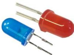
Red and blue LEDs. The short leg is the negative leg. There is also a flat side to the rim of the bulb; this will also indicate which side is negative.
