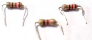
Three resistors. Check the coloured stripes - the two identical ones are 220 Ohms and the odd one out (with a blue stripe) is 4700 Ohms. The more Ohms, the more resistance to electricity. Resistors can be placed either way around.
