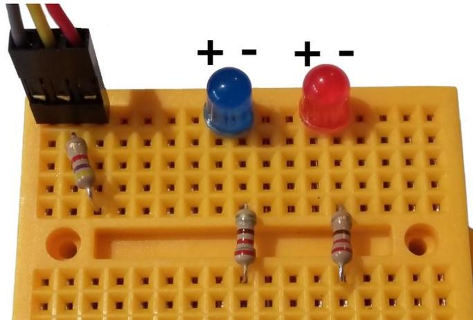
The 4700 Ohm resistor crosses the columns between the temperature sensor's data connector (centre), and the positive connector (right).
